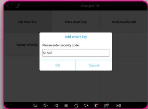
**7.** Following the instructions show on the screen, hold the key close to the start button (where the key induction coil is located), then press and hold the button within 30 seconds until the device displays the result. Press "OK" when you're ready to begin this process.
